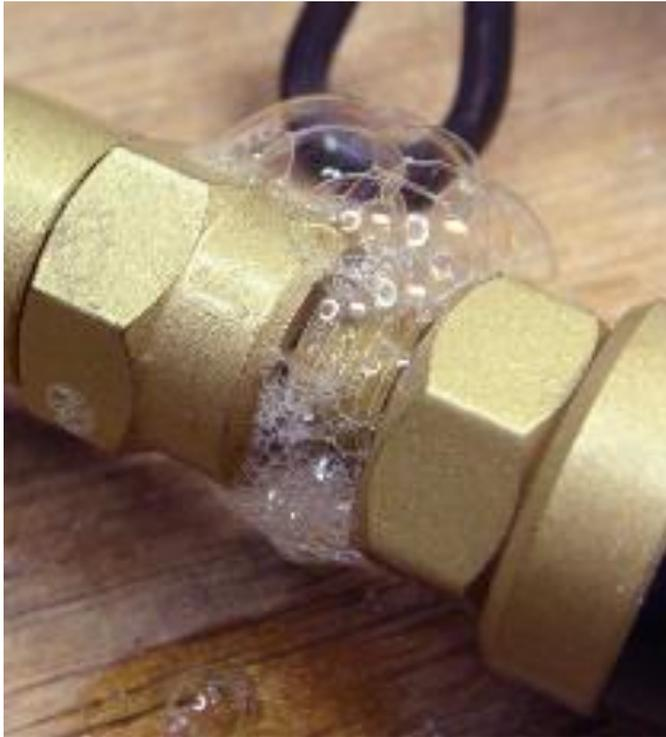
This procedure can be carried out on all connections found in the gas system. After you start with the gas bottle continue onto the gas hoses, then the regulator and slowly continue along the gas
