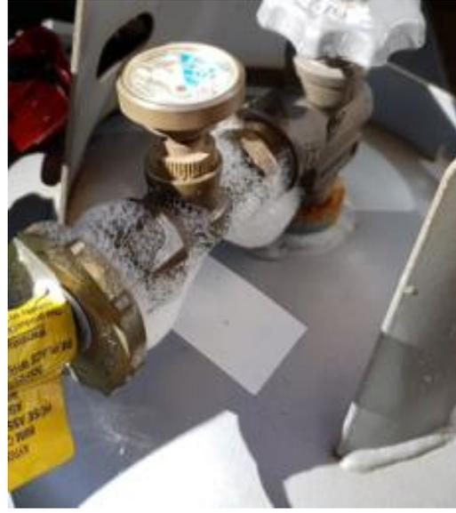
If, however you find a leak the gas will begin to create bubbles that will double and triple quite quickly. The bubbles will increase in size as they fill with gas before bursting. You may also find that you can smell the gas in the effected area.
