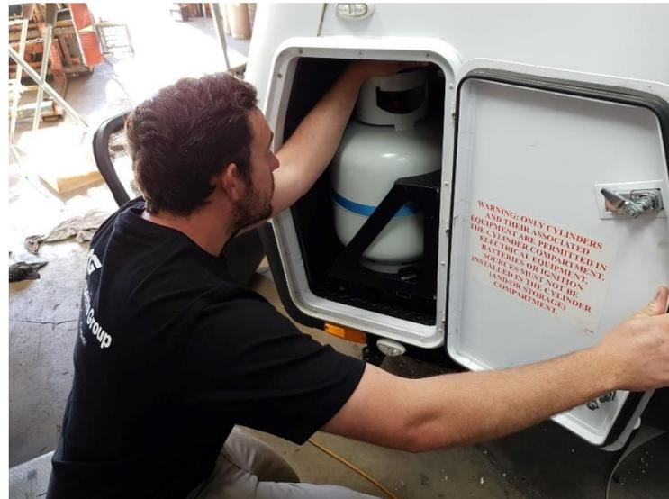
Gas bottles are also issued with an expiry date and require testing every 10 to 15 years depending on size. Always inspect your bottle for visible signs of damage or corrosion that could be hazardous to yourself or others.
